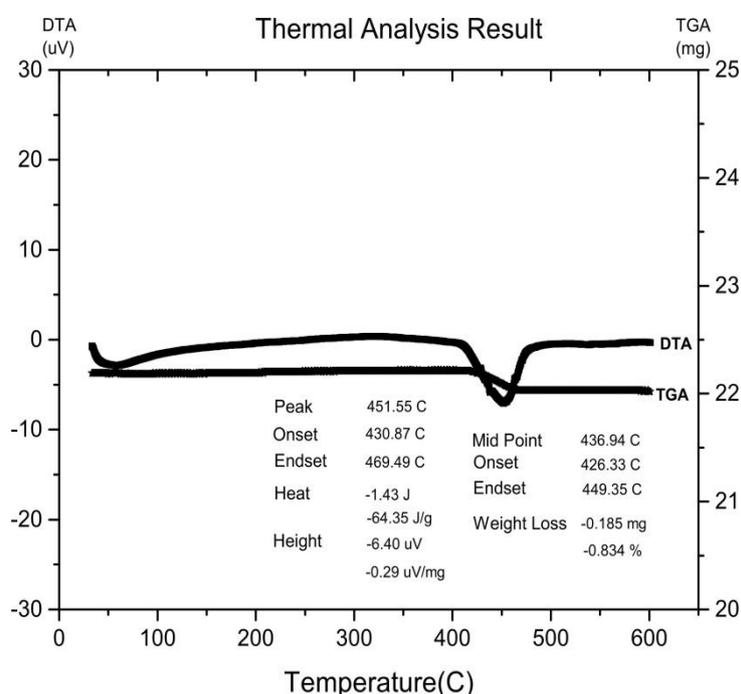
**Figure 8.** DTA/TGA for synthesized HA with a stirring time of 60 min.
