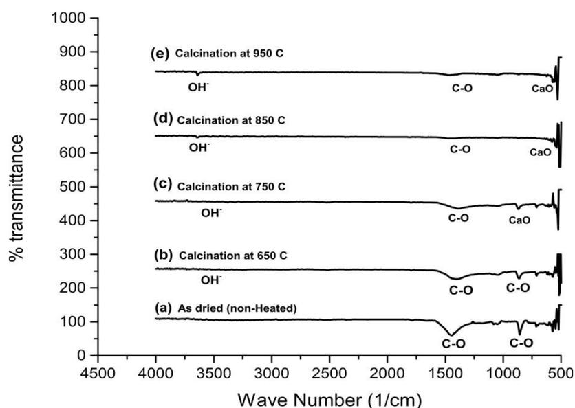
**Figure 1.** FTIR spectra of samples: non-calcination (a), calcination at 650°C (b), 750°C (c), 850°C (d) and 950°C (e).
