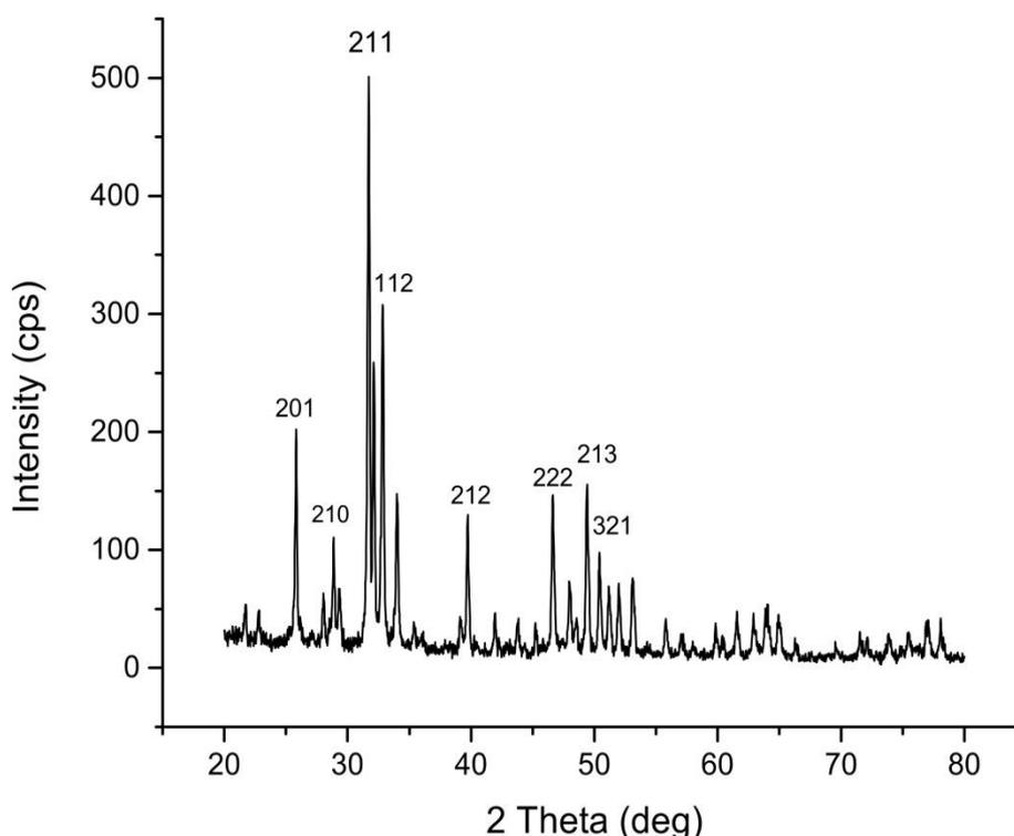
**Figure 4.** XRD pattern of the synthesized HA with a stirring time of 60 min.
