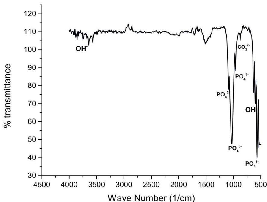
**Figure 5.** FTIR spectra of synthesized HA with a stirring time of 60 min.
