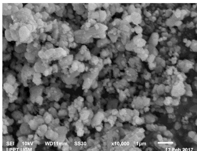
**Figure 6.** SEM images of synthesized HA with a stirring time of 60 min.
