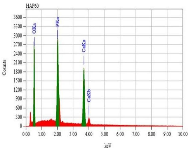
**Figure 7.** EDX analysis of synthesized HA with a stirring time of 60 min.
