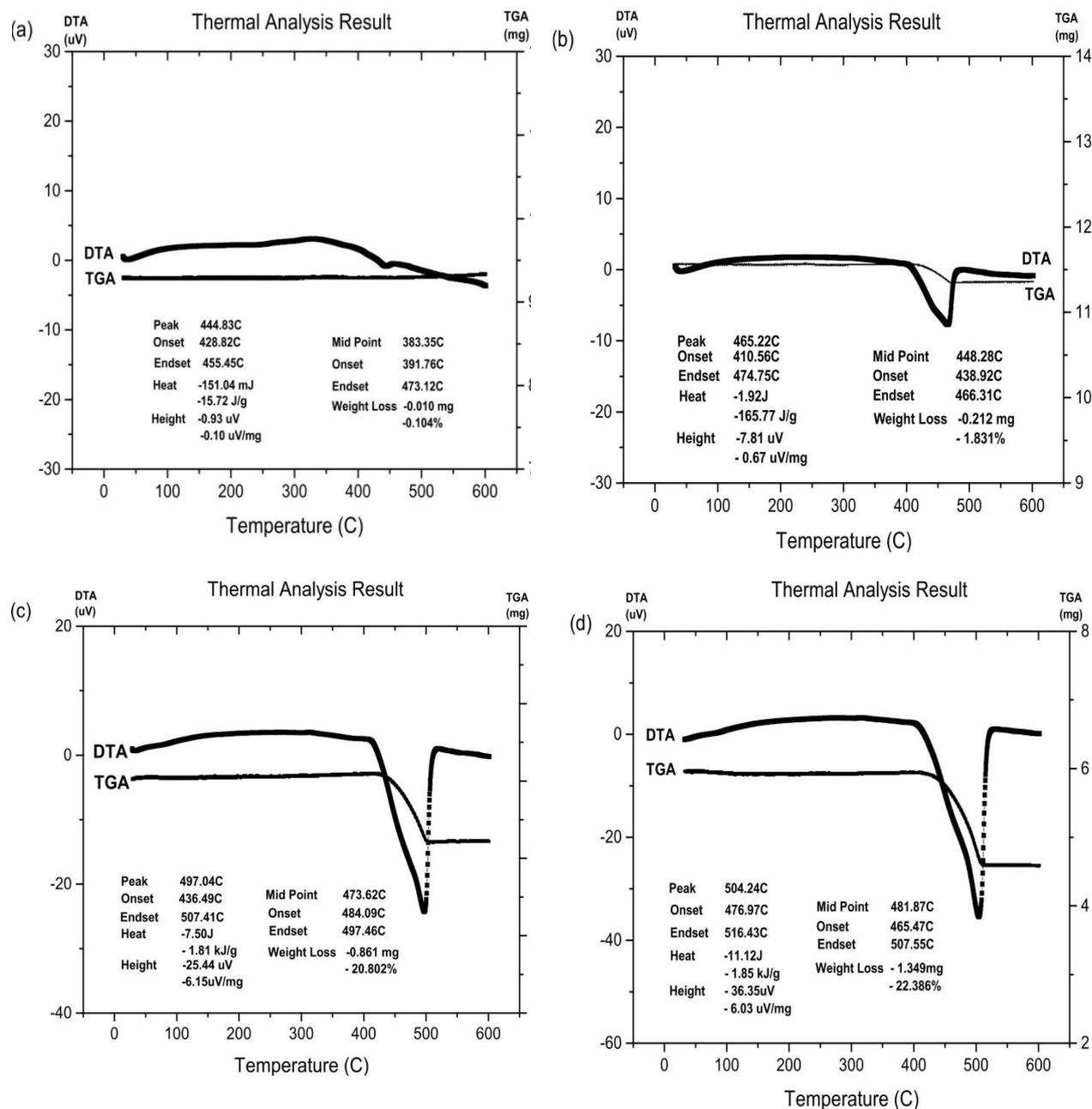
**Figure 3.** DTA/TGA results of calcium oxide at calcination temperatures (a) 650°C, (b) 750°C, (c) 850°C and (d) 950°C.
