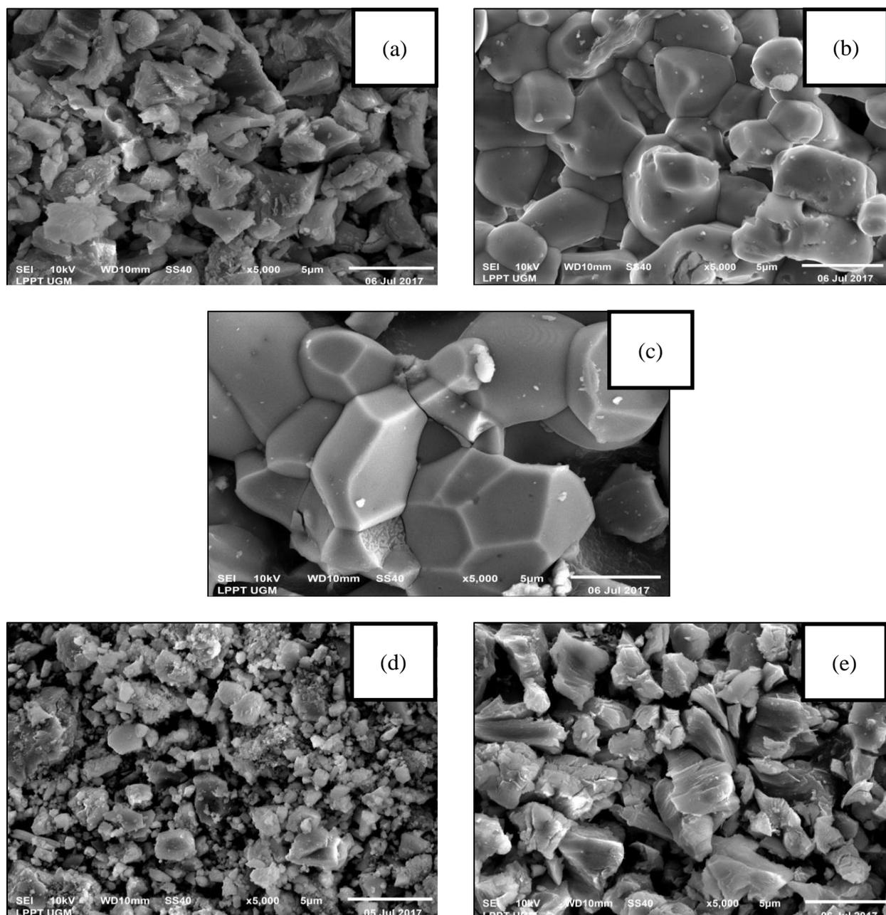
**Figure 2.** Results of SEM characterization for five samples: green mussel shells (a), calcination temperature of 650°C (b), 750°C (c), 850°C (d) and 950°C (e).
